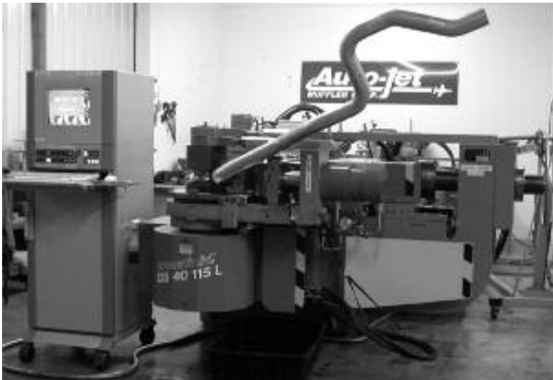
Actual photo of Auto-Jet's "Custom Designed" Tube Bending Tool
